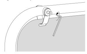
Locate panel onto the panel hanging clips. Reassemble the panel hanging clips using the screws and fixings.
